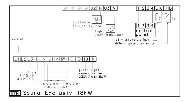
The electronic control is fused on the circuit board by a 0.16A fine fuse. In the control device there is a 16A fuse for ventilator and light. The sauna heater is not protected against short-circuit. The short-circuit protection has to be ensured by suitable constructional fuses (max. 32A).
